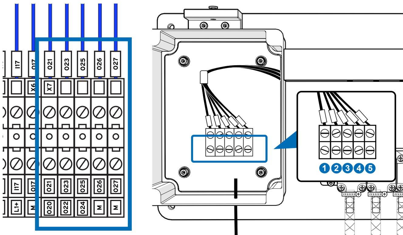
Use a 7x1mm<sup>2</sup> cable for the connection between the control cabinet and the distributor. Connect the distributor to terminal block X7. Each terminal connection corresponds to the outlets numbered from left to right, with the number dependent on the order. Below is the wiring diagram for the main unit.
