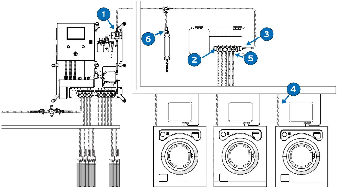
To connect equipment, distributor and washers, use **10x16 braided PVC pipe** and stainless steel clamps.
