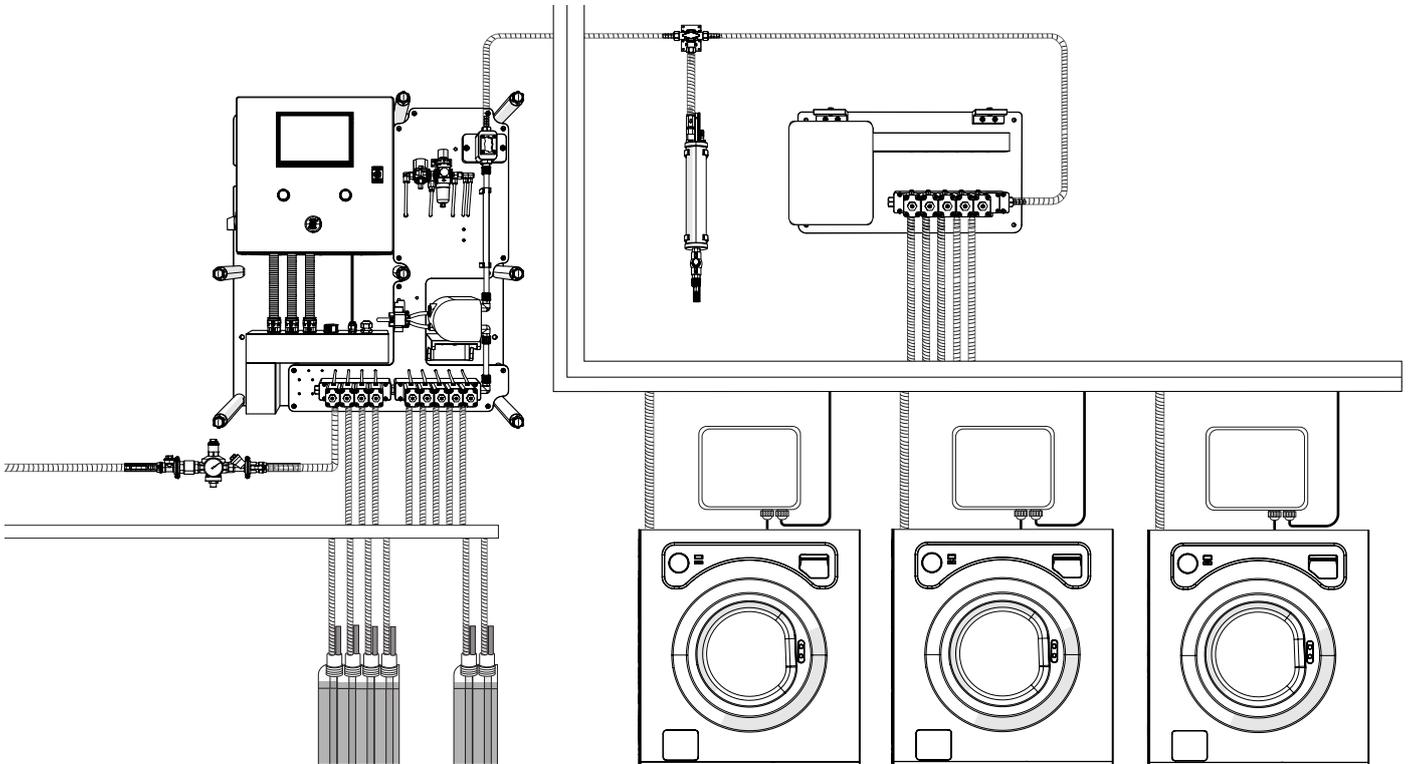
This image reproduces the 'Standard' setup of a Multiplex unit with one channel, understanding "Channel" as a group of products that are injected into the same manifold and directed to a distributor (washing machines) or an injection (tunnel).
