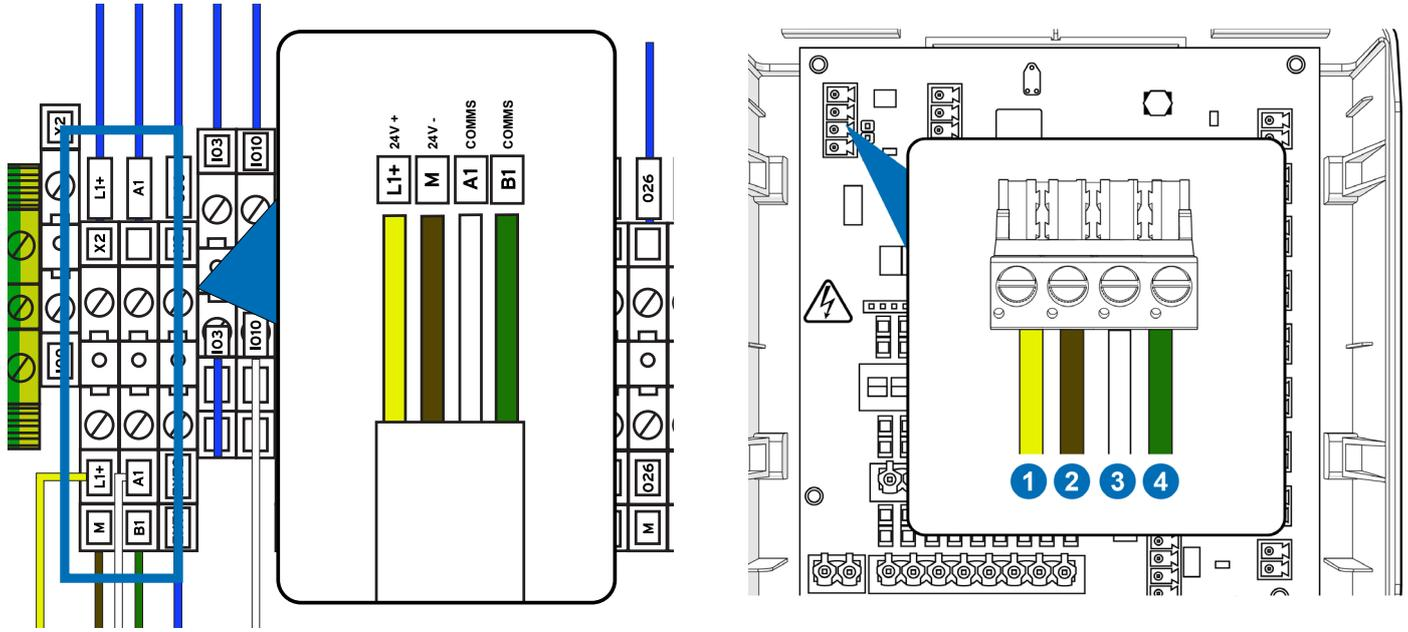
To connect the external communication box to the unit, connect terminal X2 on the main machine to terminal X1 on the communication box. Each communication box can serve up to two washing machines.
