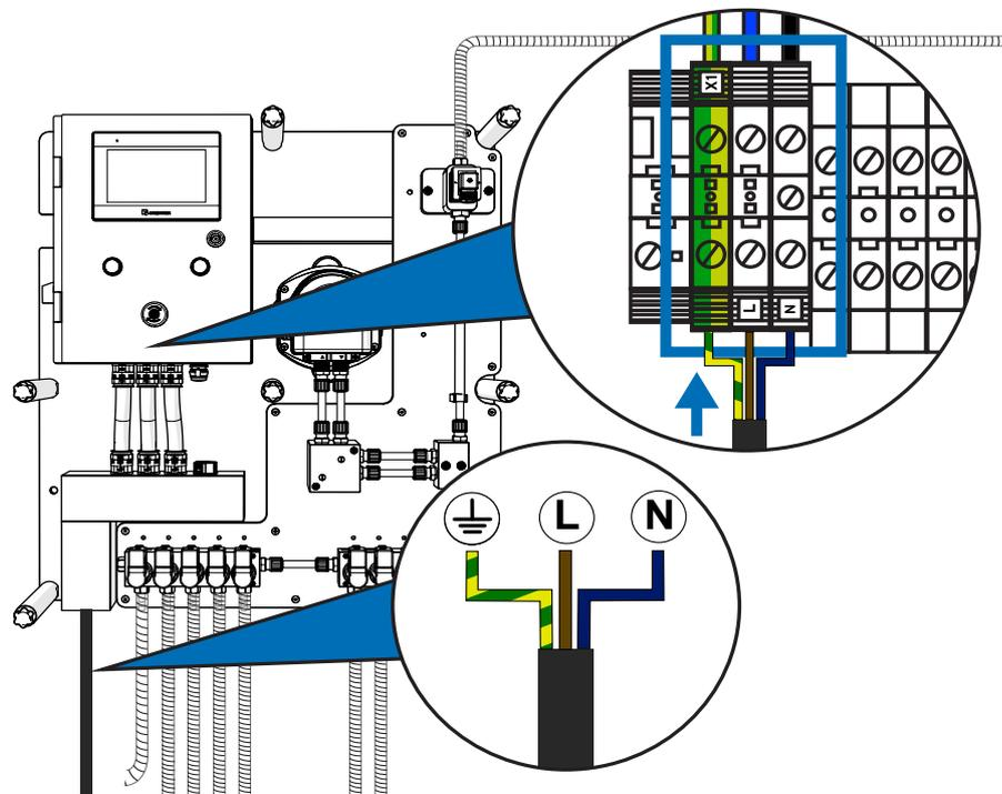
For the power supply of the equipment you must use **3x1'5mm<sup>2</sup> cable**. Insert the cable through the channel located at the bottom left and use one of the cable glands to insert it safely inside the control cabinet. Connect to the terminals identified with **X1** found on the lower left of the connections.
